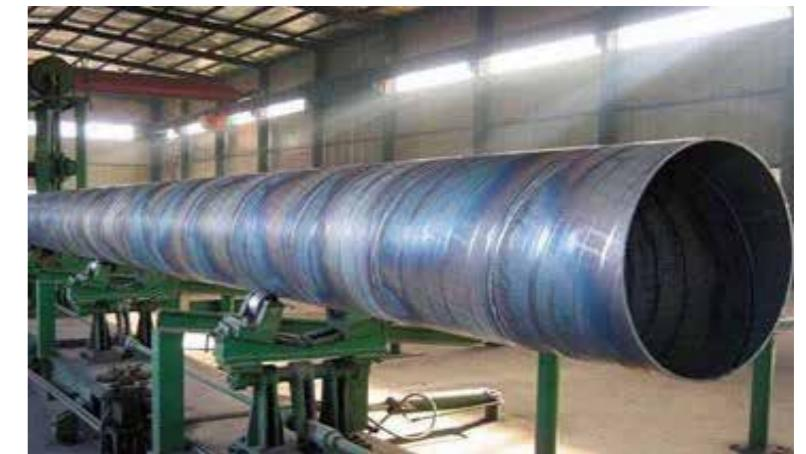
The spiral submerged arc welded pipe (SSAW) is a steel coiled pipe whose forward direction has a forming angle (adjustable) with the center line of the forming pipe, and is welded while forming, and its weld seam is formed into a spiral line. The advantage is that the same specification of strip steel can be produced. The steel pipes of various diameters and specifications have a relatively large range of raw materials, the welds can avoid the main stress, and the stress is better.
